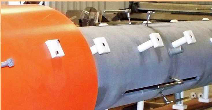
Channel 13 top mount slot antenna
